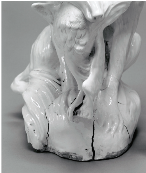
Fig. 5. Firing cracks in porcelain animal. "Fox with a Chicken," Johann Gottlob Kirchner, ca. 1732, J. Paul Getty Museum (2002.47). Height, 46 cm (18 in.); width, 34 cm (13 \frac{3}{8} in.); depth, 20 cm (8 in.). Courtesy of the Decorative Arts and Sculpture Conservation Department, J. Paul Getty Museum.
