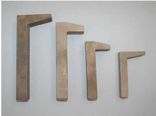
Fig. 3. Cast bronze clips in a range of sizes. Courtesy of the Decorative Arts and Sculpture Conservation Department, J. Paul Getty Museum.
