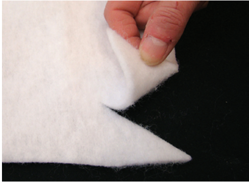
Fig. 2. Fosshape 600 in its raw or untreated state. It is a felt-like material that can be cut easily with a scissors and sewn by hand or machine in both its raw and hardened states.
