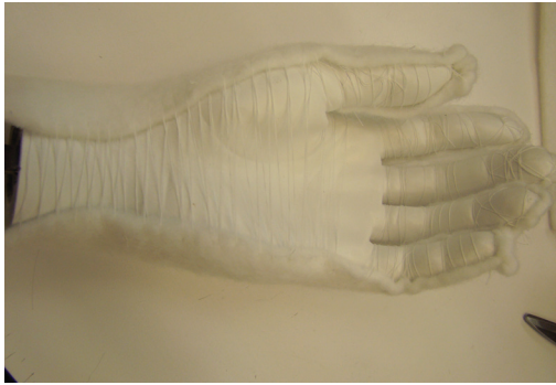
Fig. 14. A mannequin hand covered on the top only with Fosshape. The material is secured across the palm with thread and ready for steaming.
