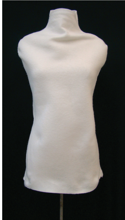
Fig. 3. A machine-sewn, baggy Fosshape 600 form pulled over a standard small-size dress form in preparation for application of steam heat, which will shrink the material to the form.
