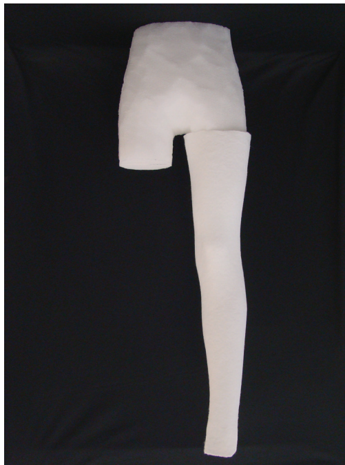
Fig. 9. An elongated torso form is carved from polyethylene foam with leg extensions to which one leg has been attached. The polyethylene form will be glued into the bottom of the Foshape torso.
