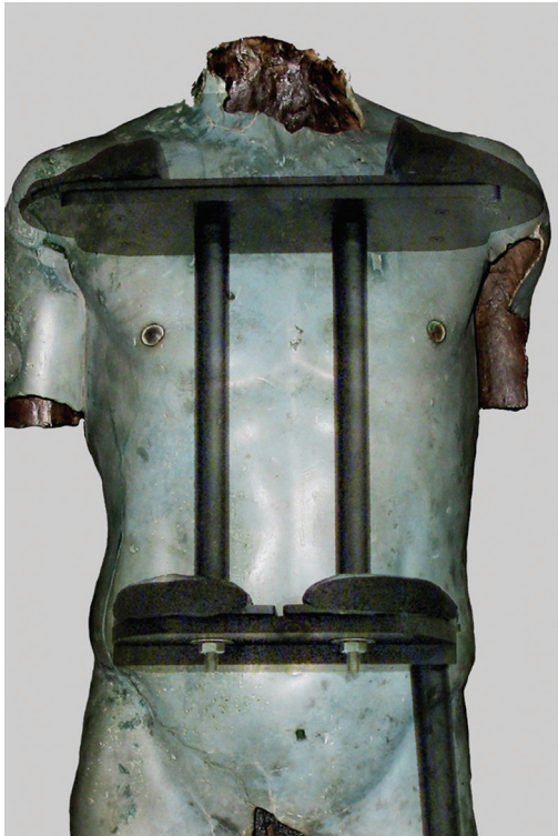
Fig. 8. Detail illustration showing the connection of the shoulder support to the midlevel support, superimposed on the image of the torso.
