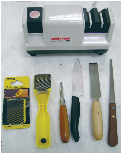
Fig. 13. Some tools used to carve and finish the mannequins. Electric knife sharpener (for steel blades only) at top, lower row (left to right): Surform rasp and replacement blade, burnishing tool for inserting material into Ethafoam (fig. 14), ceramic knife, steel square-edged knife, and steel pottery knife.
