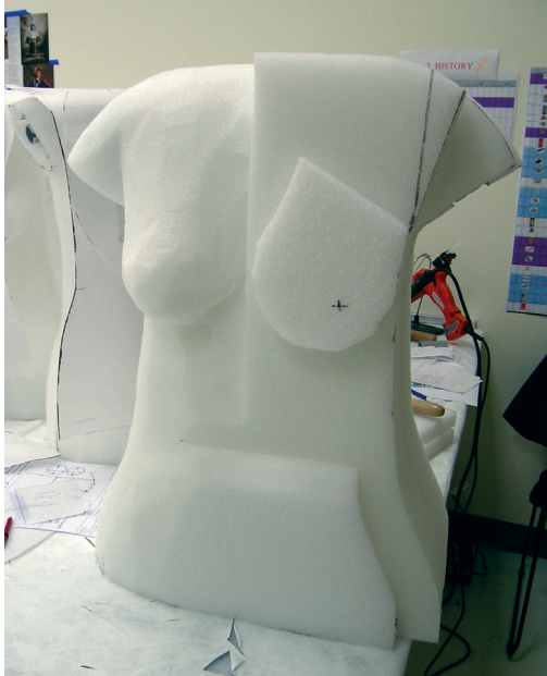
Fig. 9. Partially carved Ethafoam mannequin demonstrating block construction with planks of various thickness of foam.
