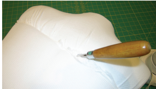
Fig. 14. Demonstrating the use of the burnishing tool to insert stockinette into a slit in the Ethafoam.
