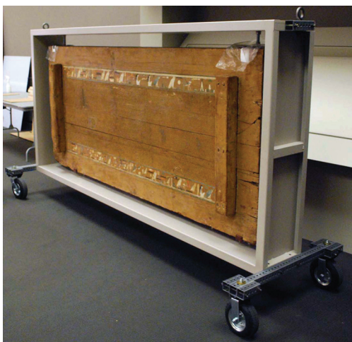
Fig. 12. The coffin lid, mounted into its new frame, can now be transported easily through the museum with the use of a temporary pneumatic travel wheel system.
